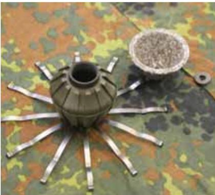
Testing found 98 percent of blast fragmentation from the new AB HGr to be found within a 5m radius © AJB
