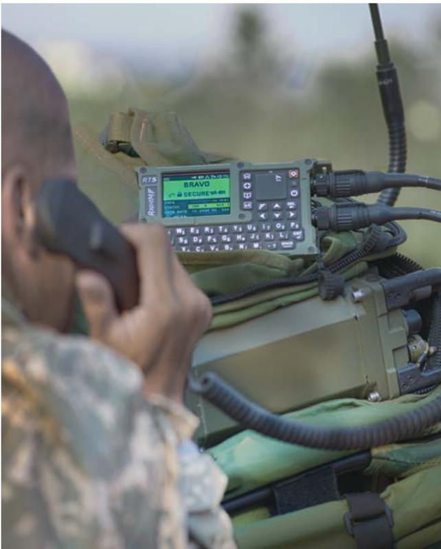
RT5 in secure voice usage, interfaced to a tactical radio.
