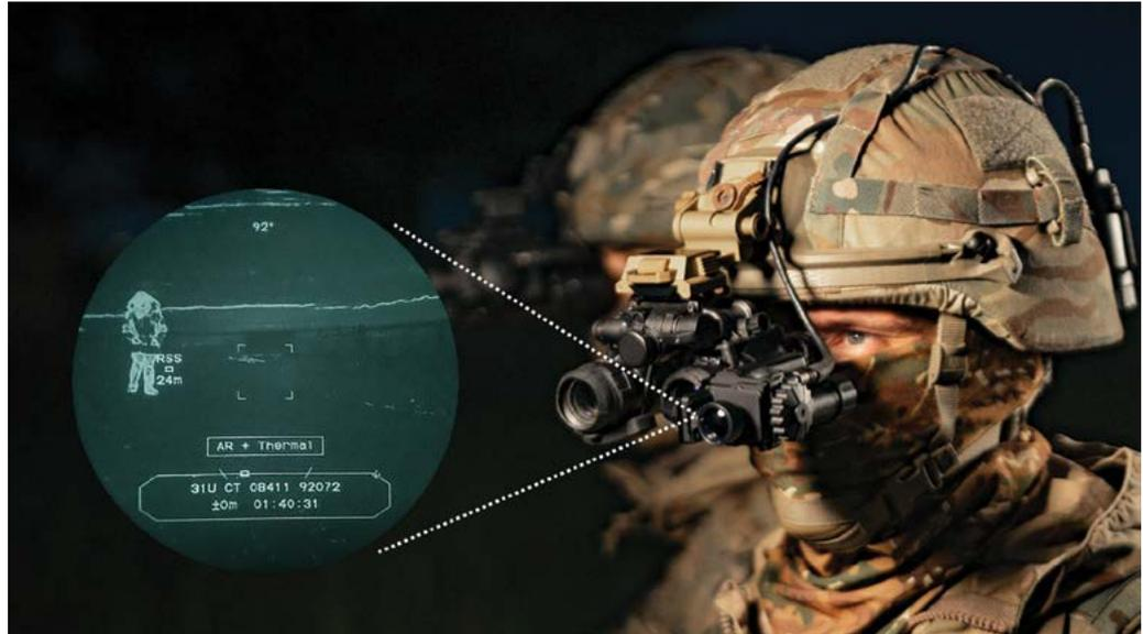
Augmented reality (AR) and operational data is overlaid on the clip-on thermal imager viewer.
