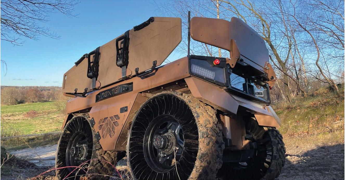
UGV using Bren-Tronics 6T battery. Nexter robotic ©
