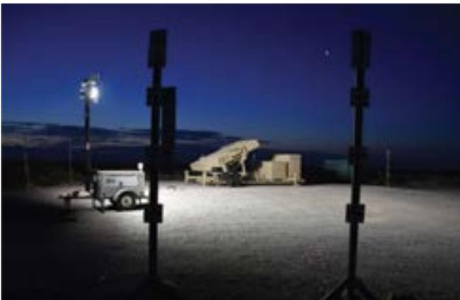
*The Indirect Fire Protection Capability Increment 2 is a mobile, ground-based system designed to defeat subsonic cruise missiles, Group 2/3 unmanned aircraft systems, rockets, artillery, mortars and other aerial threats. (Heriberto Ibarra WSMR)*
