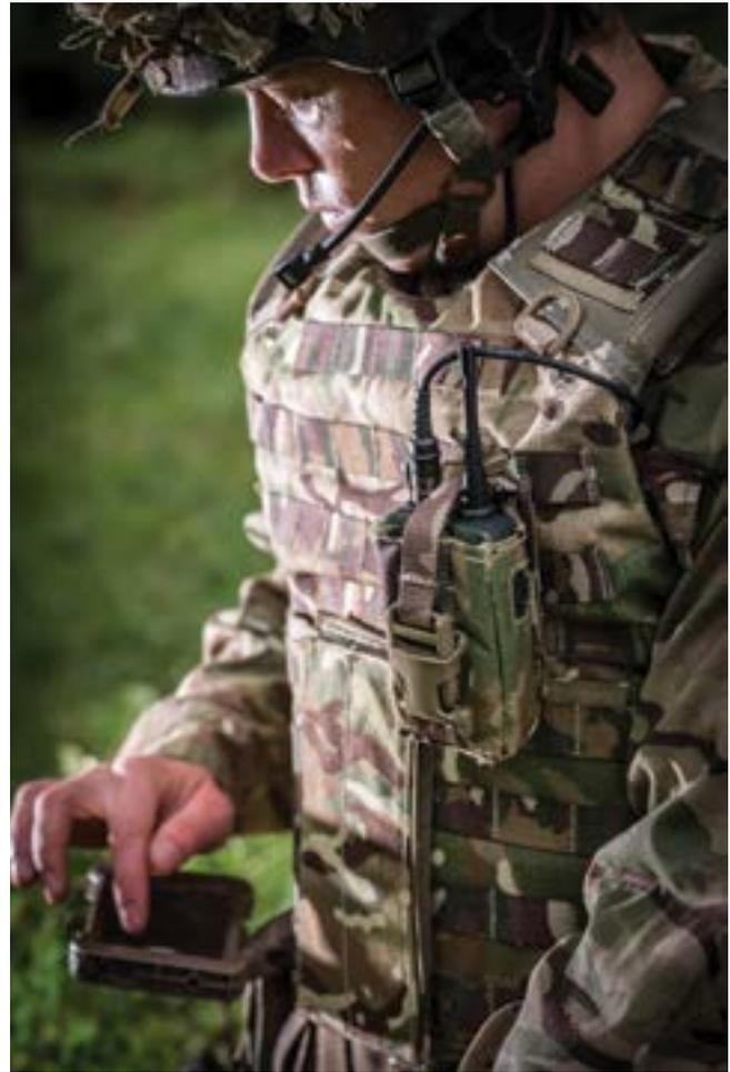
The radio holds 100 pre-set channels so a user can select the mix of services required by changing channel.
