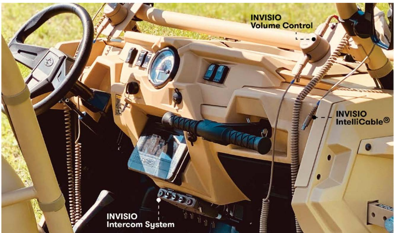
The INVISIO Intercom system is easy to install in e.g. light tactical vehicles due to its size and weight.
