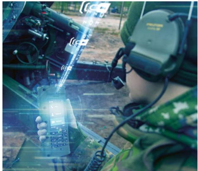
*The Tough Comnode device fulfils the data transfer and communication needs for mobile troops for example as a SIP phone, router and SHDSL modem. (Image: Bittium)*
