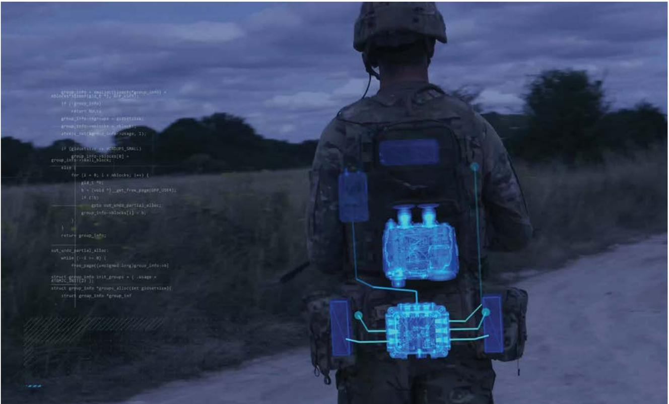
The Thales SHArc showing the hub attached to two batteries, a tactical radio, and other connector points with other data enabled but currently unattached devices in a stored position.
