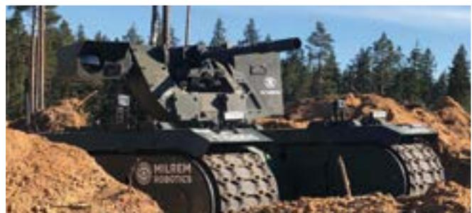
deFNder® Medium remote weapon station fitted with FN® M3R machine gun, on UGV
