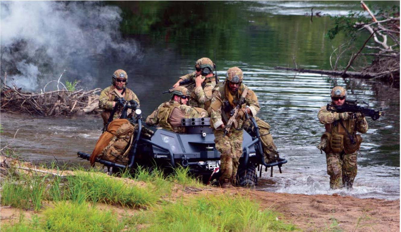
*Argus can control the Mission Master UGV and receive data from its many sensors. Using the "follow me" mode, the UGV can roll alongside other soldiers, who can ensure the area is secure.*
