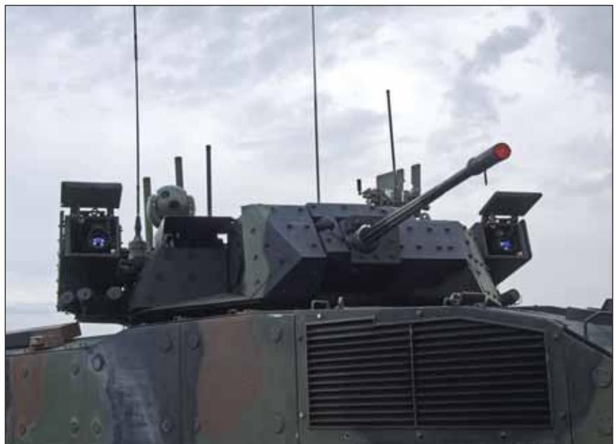
*The turret of the antitank version of the Freccia is equipped with the Janus independent commander's sight which will also equip the company commanders' vehicles. © P. Valpolini*
