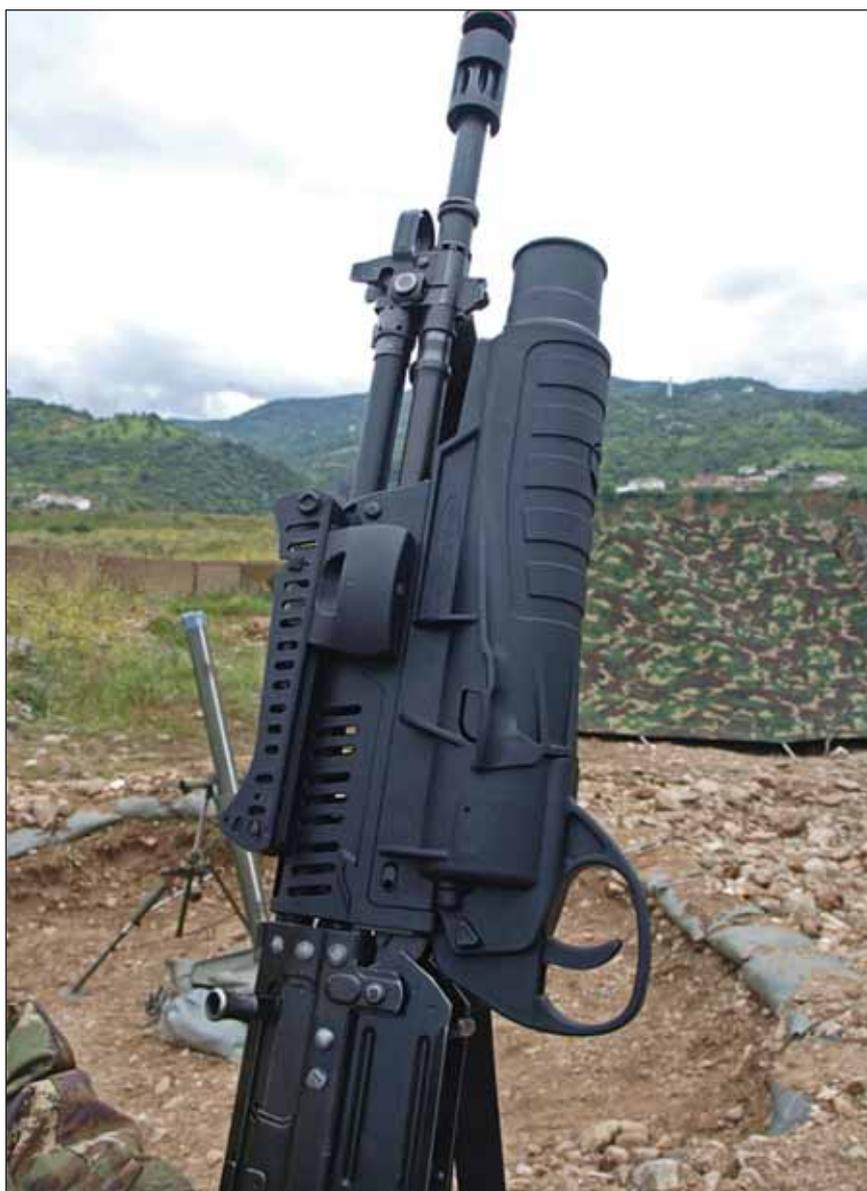
The Beretta GLX-160 grenade launcher has been adopted by the Italian Army which is using it on the Beretta 70/90 rifle; a special interface is used to attach it to the weapon. © P. Valpolini
