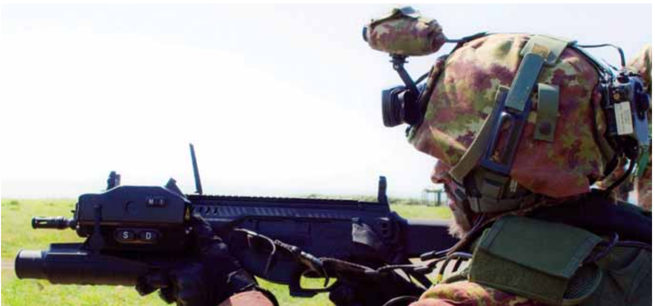
SCORPIO's ballistic computer, re-configurable for selected ammunitions, provides an enhancement of the hit probability against stationary and moving ground targets. © SELEX Galileo.
