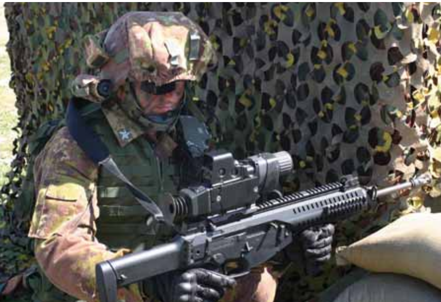
The ASPIS rifle sight features aiming laser pointers for close combat operations and uncooled infrared, day TV, and "shooting around the corner" video outputs transmitted to the soldier by wireless technology. © SELEX Galileo.
