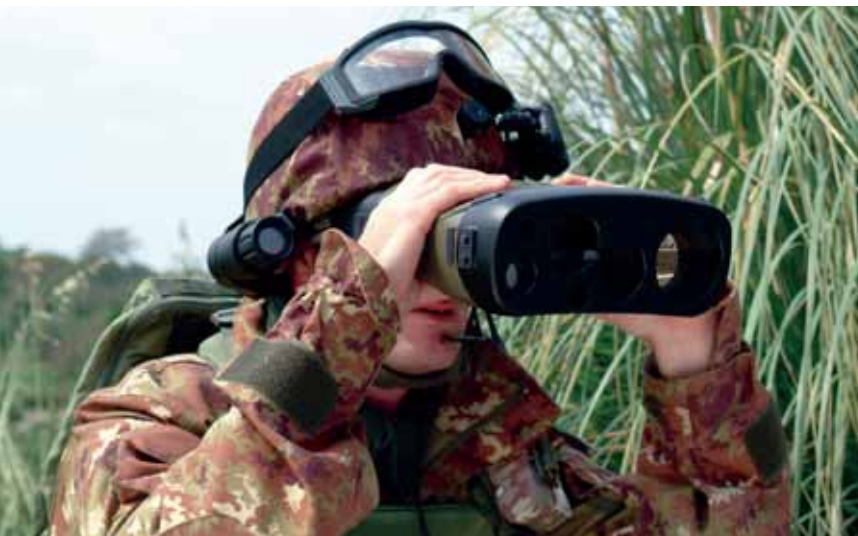
Linx is a hand-held target locator which includes an uncooled thermal imager for all-weather observation and detection, day optical telescope, eye-safe range finder and digital compass in a lightweight unit. © SELEX Galileo.
