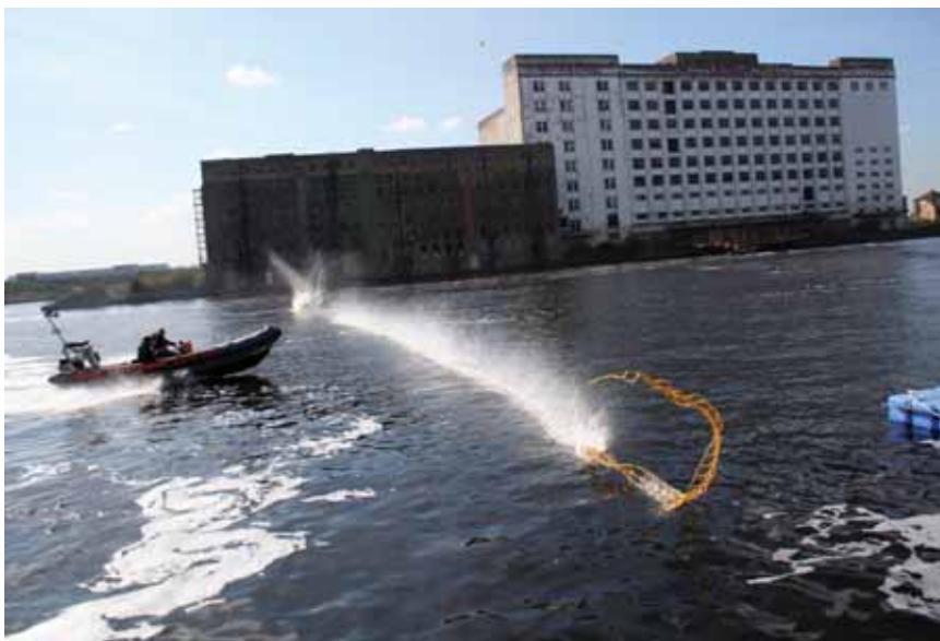
A 60 metres floating vessel entanglement line is deployed by a "Buccaneer" launcher. © BCB.
