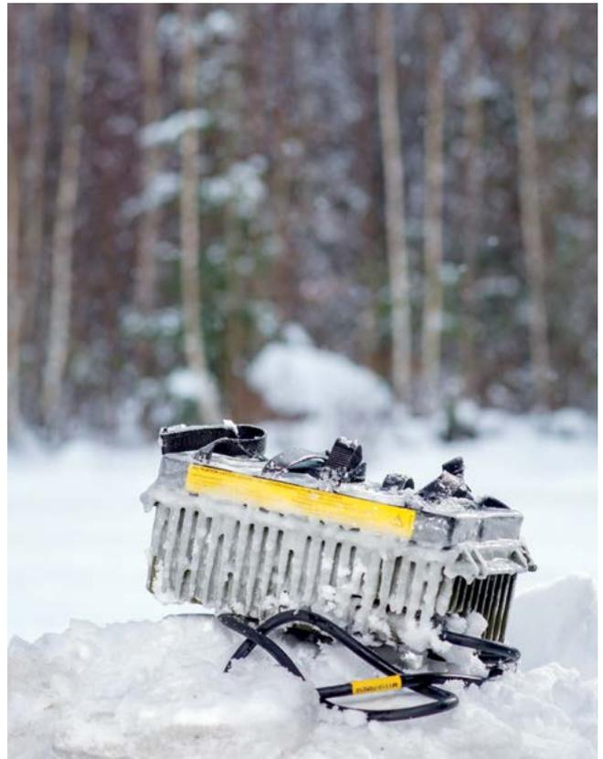
ML334-4A-24 multi-chemistry 4 channel charger. Operating in -40C temperatures.
