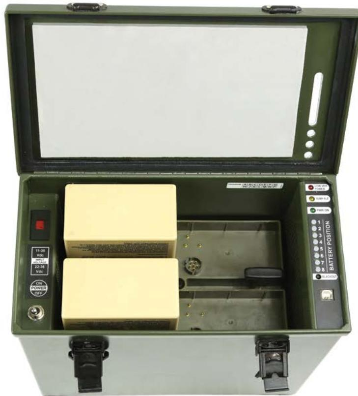
profiles can be downloaded for charging capability evolution. As of today, more than 70 different types of military battery packs are supported by Bren-Tronics Universal Chargers.
