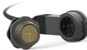
*The development of the Fischer LP360™ connector, the first product in the brand new Fischer Freedom™ Series, has introduced a new approach to connectivity, and innovative engineering and technology in mating (360° mating is possible because the LP360™ has no key code), in locking (sealed ball-locking mechanism with variable pre-defined force), and in materials (membrane-sealed contacts).*
