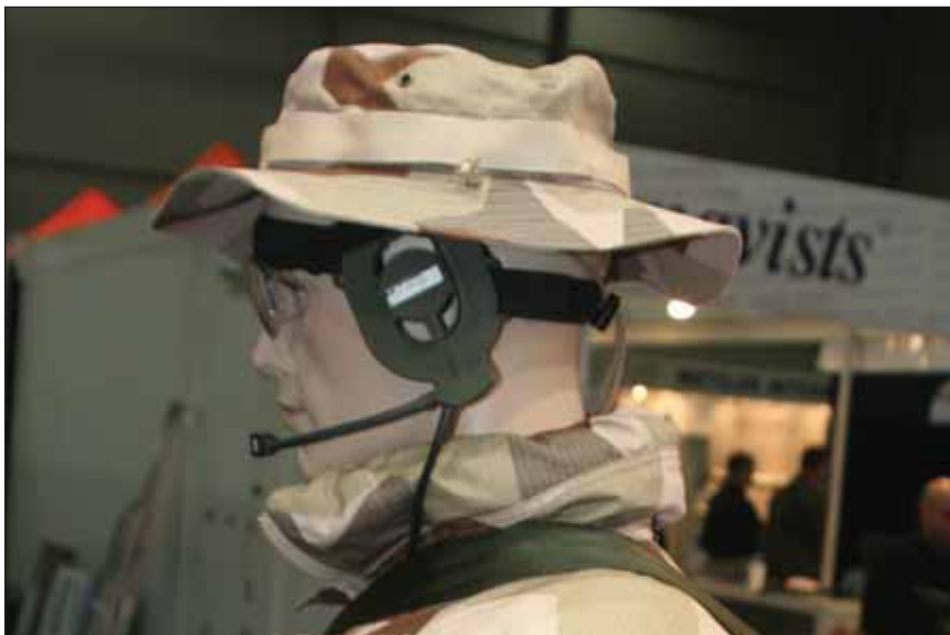
Sweden has opted for and fielded the Selex Communications H4855 PRR, designated the RA 1031 © AJB
