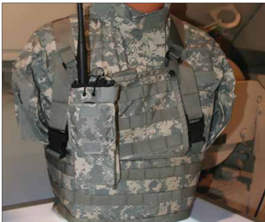
Thales Communications, Inc. is now offering its STORM family of lightweight, wearable/hand-held IED “inhibitors”. It was purposely designed to resemble Thales Communications’ hand-held (0.87-kilogram) PRC-148 Multi-band Inter/Intra Team Radio, which is in wide use by US and allied forces © AJB
