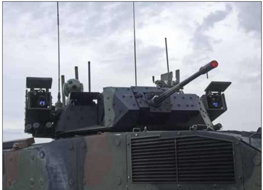
The turret of the antitank version of the Freccia is equipped with the Janus independent commander's sight which will also equip the company commanders' vehicles. © P. Valpolini
