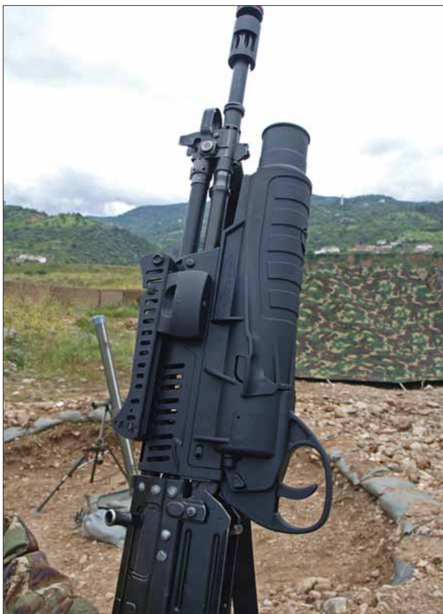
The Beretta GLX-160 grenade launcher has been adopted by the Italian Army which is using it on the Beretta 70/90 rifle; a special interface is used to attach it to the weapon. © P. Valpolini
