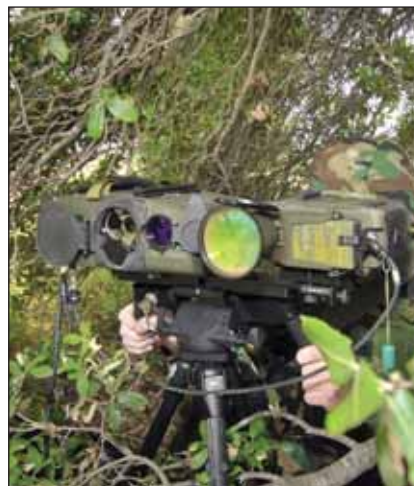
The company's "flagship" next generation PLDR weighs 5.5 kg and designates to ranges of 10 km
