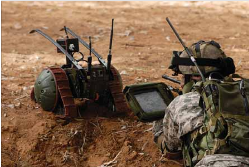
VIPeR® (Versatile, Intelligent, Portable Robot) is a small, lightweight, one-person portable robot
