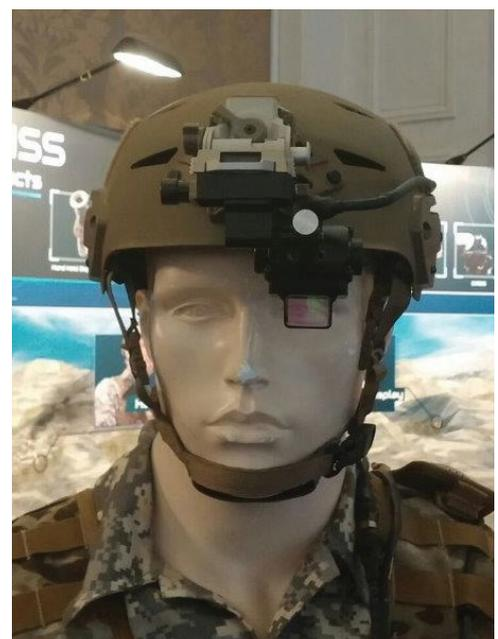
Figure 6: See Through – Helmet Head Up Display. Photo: © DMSS Group.
