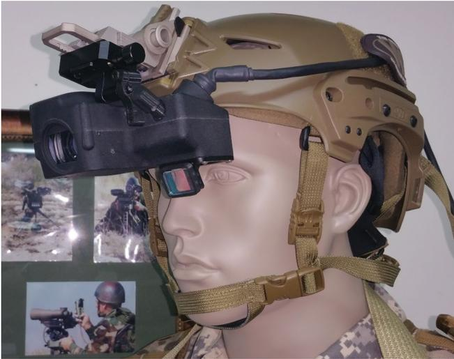
Figure 5: Near Eye Display. Photo: © DMSS Group.
