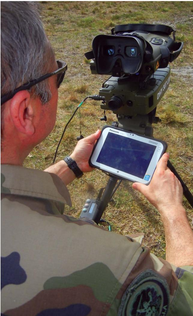
*Sagem JIM LR (Infrared Multifunction Binocular - Long Range) as the key component of a tactical targeting system which combines Delta Suite software (Impact company) and a DHY 307 LW laser designator by Cilas. The system is displayed at the last SOFINS 2015 special forces forum (Bordeaux, April 14-17 2015). Photo: © Sagem.*
