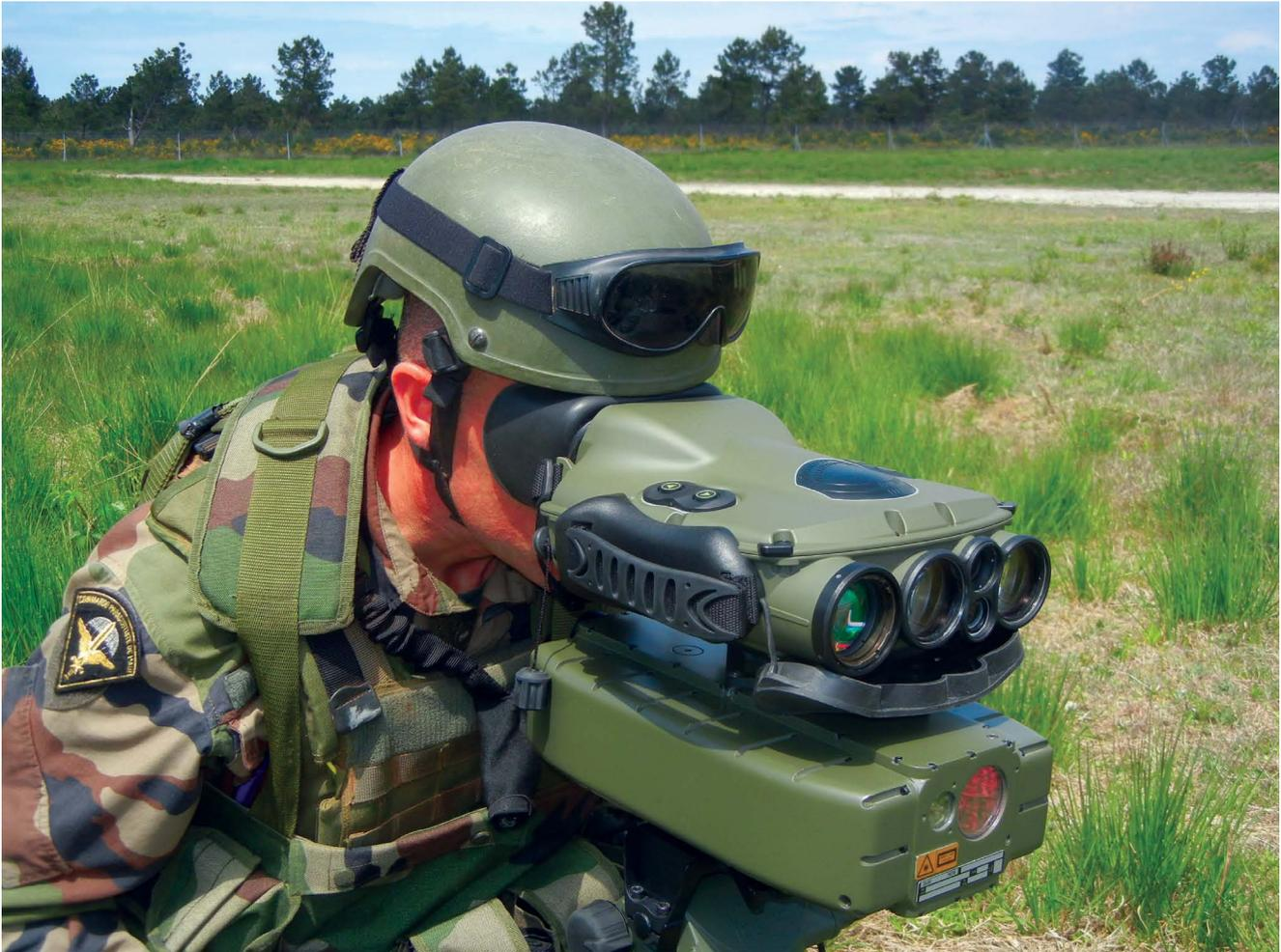
Sagem JIM LR thermal binocular can be used day or night with the new DHY-307 LW laser designator by Forward Air Controllers in "sensor to shooter" digitized loop for close-air-support missions. Photo: © Sagem.
