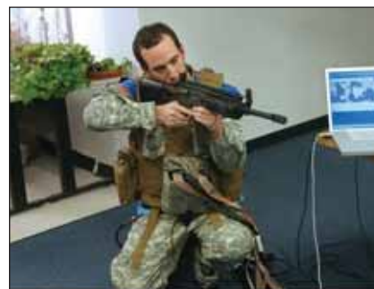
Soldier and rifle with vest and body armour being tested by Tactilus sensor system
